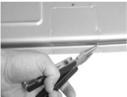
FIGURE 11 REMOVING CONDENSATE KNOCKOUT
